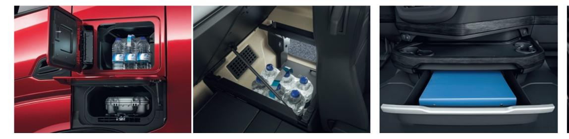
The outer compartments offer a massive storage capacity of up to 380 litres.
