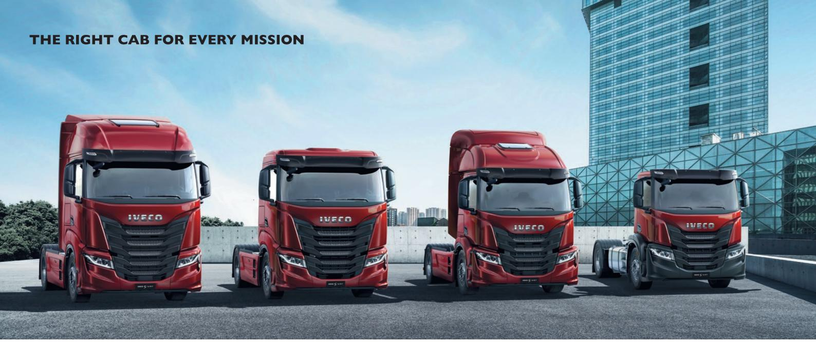
The IVECO S-WAY cab line up offers a choice of cabs to match your mission: the AS sleeper cab, the AT sleeper cab with low or medium roof, and the AD short cab with low roof.
